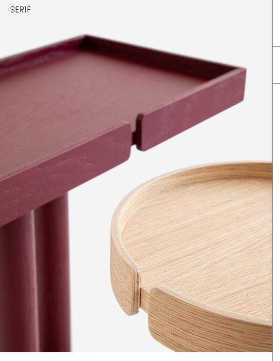
Top/base Plywood with oak veneer on both sides; the edges are made of bent plywood with double-sided oak veneer
